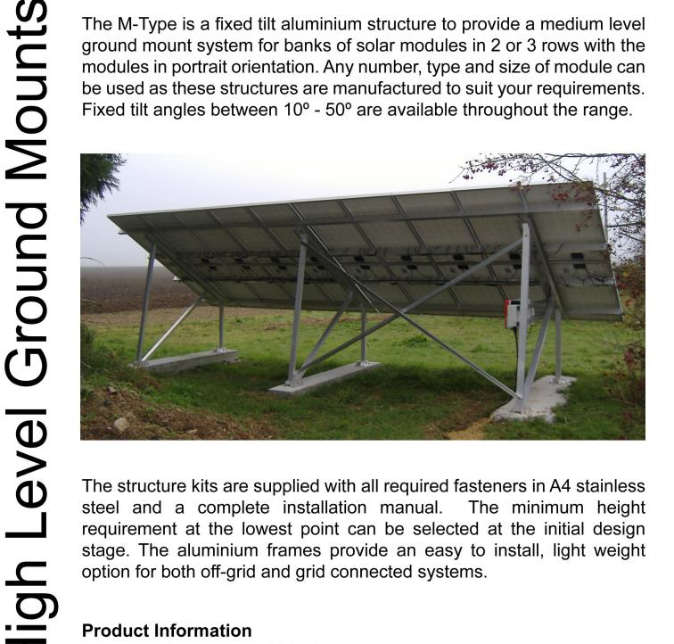
The structure kits are supplied with all required fasteners in A4 stainless steel and a complete installation manual. The minimum height requirement at the lowest point can be selected at the initial design stage. The aluminium frames provide an easy to install, light weight option for both off-grid and grid connected systems.
