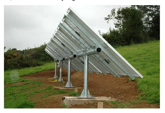
A simple foundation is required for each leg, and the slotted base plate allows for 20° of horizontal rotation for easy positioning. The structure is supplied with all fasteners and an installation manual. An optional foundation kit can be supplied prior to delivery, which includes a set of ground anchor rag bolts and a wooden template. This allows the foundations to be prepared in advance, minimising installation time.
