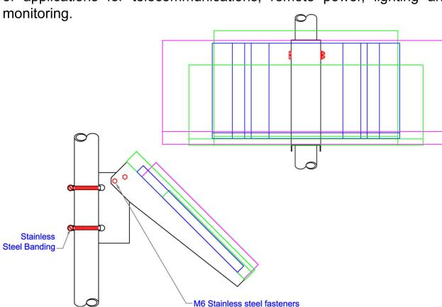
The kit is supplied complete with an installation manual, and all fasteners required to allow for the different types of solar module. Pole mounting is achieved with stainless steel banding to allow for flexibility of pole diameters from 40mm to 105mm. Wall or horizontal mounting can also be achieved using the two M8 holes provided.
