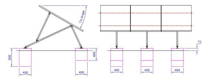
Leg lengths can be easily shortened as required by cutting the poles on site. The whole structure can be assembled with the modules face down making it easier to assemble and pre-wire without the risk of high voltages being present. Even the tilt angle can be preset, so the structure can be turned over and bolted down. The tilt angle can easily be adjusted with the use of the provided hex key.
